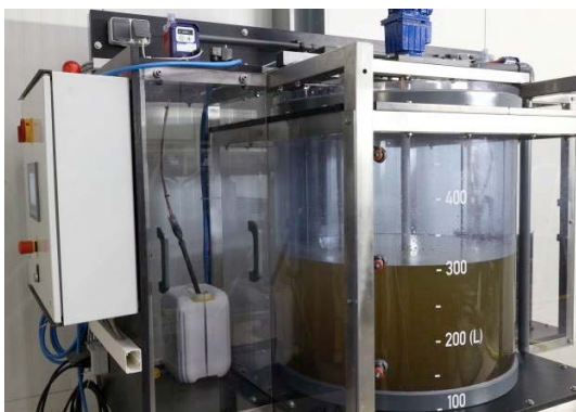
Phosphorus elimination module, 500 litre reactor and an approximately 50-litre sedimentation funnel volume
