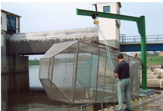
Top: Specially designed weir for quantifying the migration of young eels in use on the lower Havel
