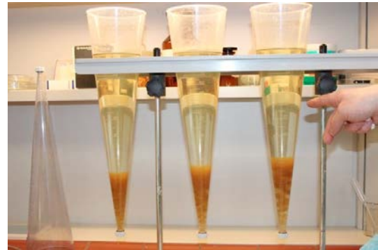
Precipitation/flocculation and sedimentation experiments in the IfB laboratory
