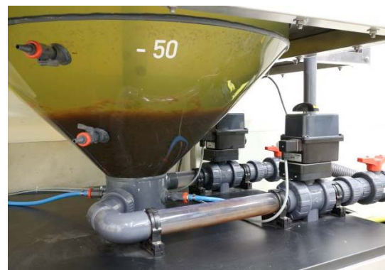
Phosphorus elimination module, 500 litre reactor and an approximately 50-litre sedimentation funnel volume
